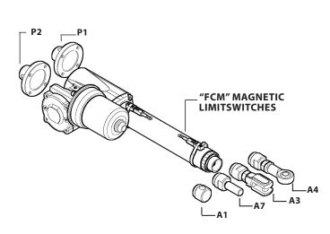
**Note:** "B" dimension changes according to model ALI3-P = see pictures ALI3-P stroke > 320 mm = + 10 mm (for all versions) ALI3-P-FCM = + 36 mm with safety nut "G" = + 30 mm Bellow + 20mm (no for versions FCM )
